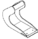
Clay Spade Buckets: Type of fittings depends on the coupling system.
