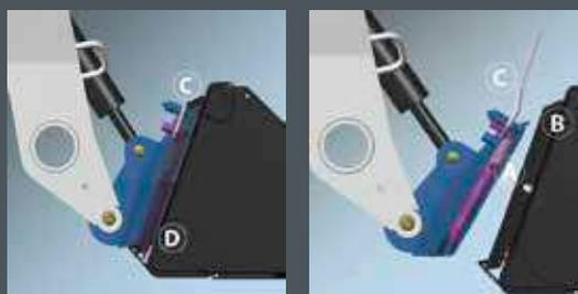
Bob-Tach™ frame (A) moves into attachment flange (B); handle (C) pushes down easily, pressing wedge (D) through frame and attachment hole for solid connection.
