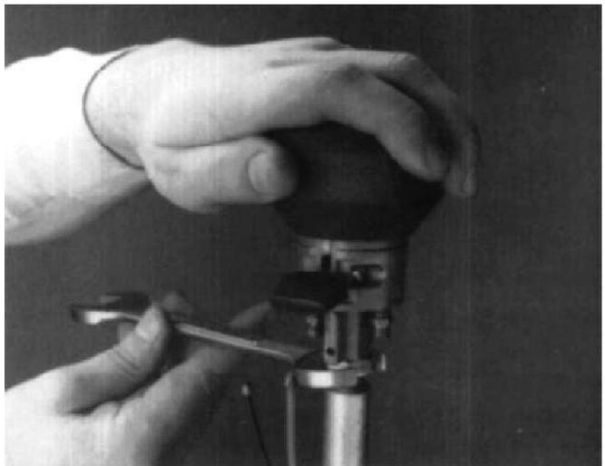
6. Connect the white air line to the "S" or Supply Port and the black air line to the "P" or End Port of the slave valve. Tighten fittings securely.
