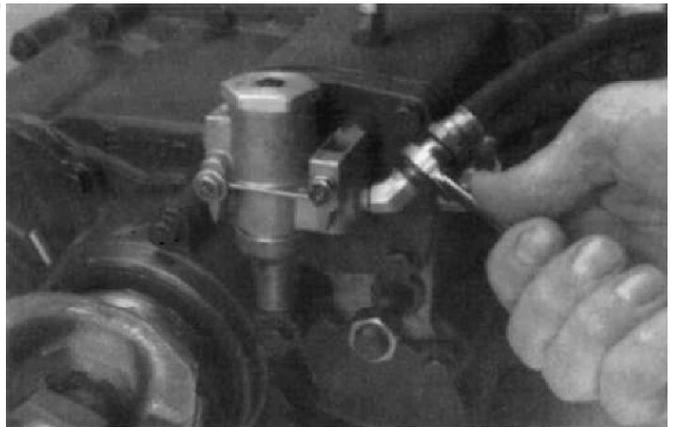
6. Remove the 2 cap screws and remove the air filter/regulator assembly.
