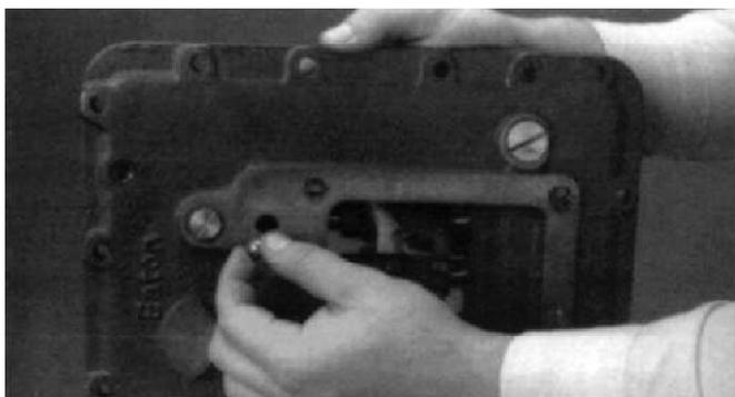
3. Tilt the assembly and remove the 3 detent balls from the housing bores.
