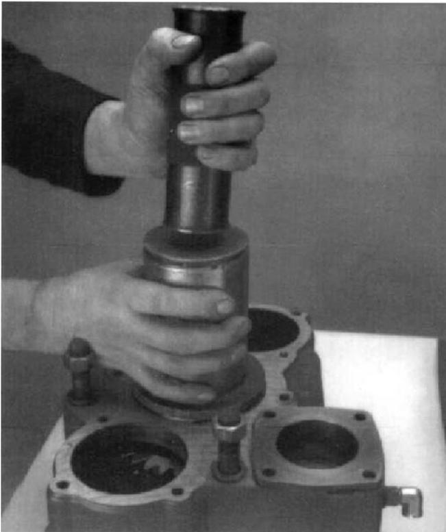
7. Install the bearing in the housing bore.
