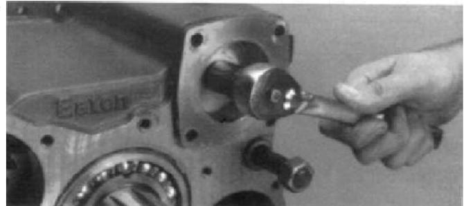
7. Install the gasket and cylinder cover with the HI Range port to the right. Tighten the 4 capscrews to the recommended torque.
