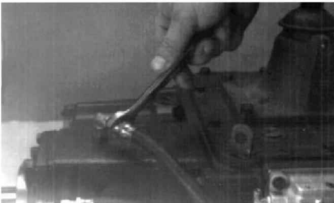
2. Connect the 1/4" I.D. air hose between the slave valve "L" port and the range cylinder "L" port. Tighten both connections to the recommended torque.
