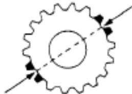
*Drive gear teeth correctly marked for timing.*
