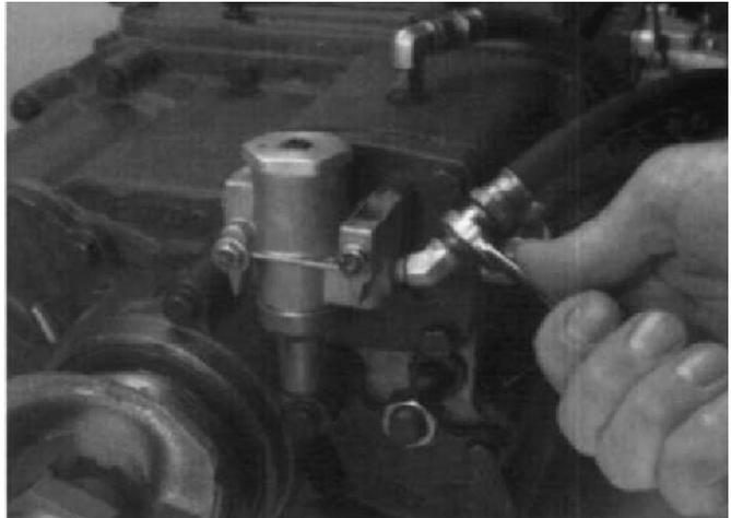
5. Install the Roadranger valve cover over the 2 air lines and gear shift lever. Install the jam nut on the shift lever. Thread the Roadranger valve on the shift lever and secure by tightening the jam nut against the Roadranger valve.
