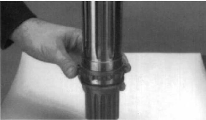
2. Place splined washer on the output shaft shoulder facing up as shown.
