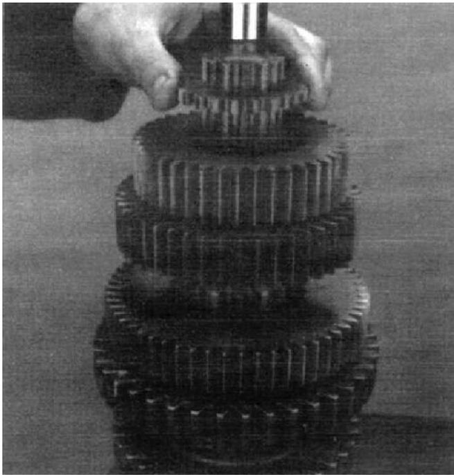
21. Install a tolerance washer in the 3rd speed gear bore.
