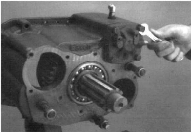
2. Remove the yoke bar nut and washer.
