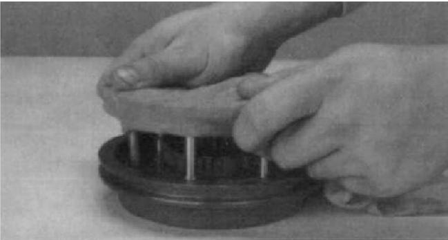
1. Place the larger LO Range synchronizer ring on the bench. Cover the assembly with a shop rag to prevent losing the three springs released from the Hi Range synchronizer at the pin locations. Pull the HI Range synchronizer from the blocker pins.
