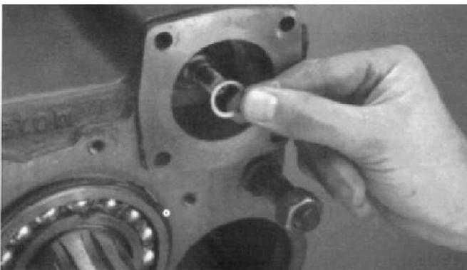
3. Install the copper gasket on the yoke bar threaded end.
