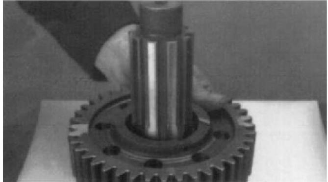
4. Install the LO Range gear rear washer on the output shaft and against gear, with the chamfer side facing up.
