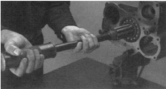
1. Using a soft bar and maul, drive or press against the output shaft rear to move assembly forward and from the rear bearing.
