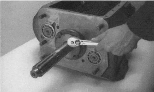
1. Remove the 4 cap screws retaining the front bearing cover. Remove the bearing cover and gasket.
