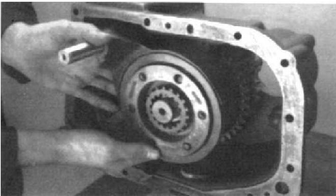
2. Place the yoke in the sliding clutch slot; threaded end of the piston bar towards the larger LO Range synchronizer. Place the entire assembly in the auxiliary housing, engaging the sliding clutch splines with the output shaft and inserting the yoke bar through the cylinder bore.
