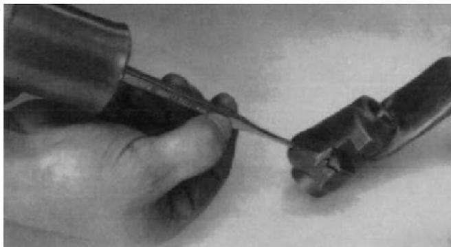
3. Place the housing in a vise with the front of housing to the right as shown. Install the 4th-5th speed shift bar in bottom bore with detent notches to the front, installing yoke, lock screw, and safety wire.
