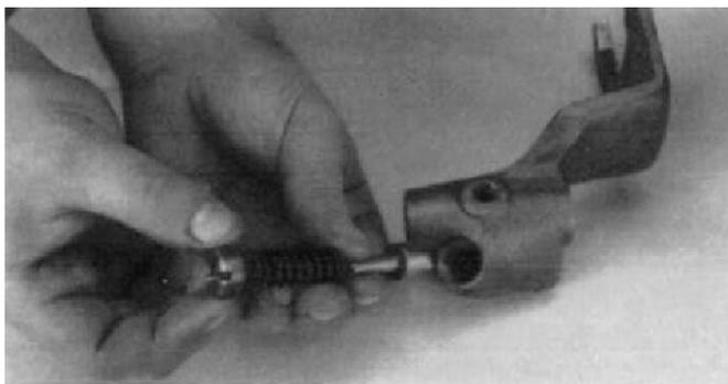
1. If previously removed, place plunger stop in 1st-reverse shift yoke block, install spring in bore of yoke and onto shank of plunger. Install the plug and tighten to compress the spring.
