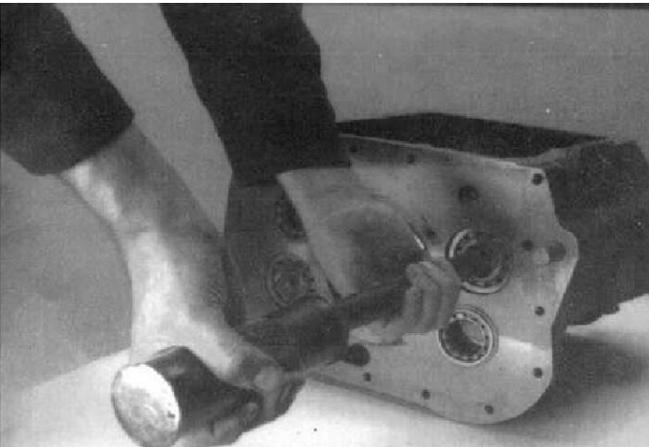
2. Use a soft bar and maul against the countershaft rear and move the countershaft assembly forward as far as possible until the snap ring groove in the front bearing is exposed.
