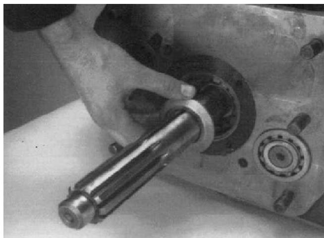
6. Remove the drive gear snap ring.
