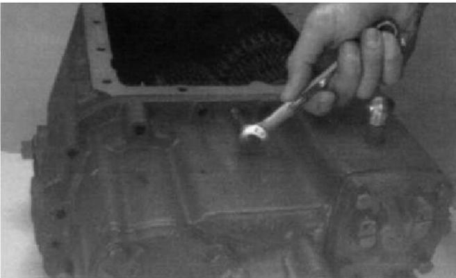
2. Insert 3 cap screws in the housing flange tapped holes. Tighten evenly to move the auxiliary section back: leave a space wide enough to attach a chain hoist.
