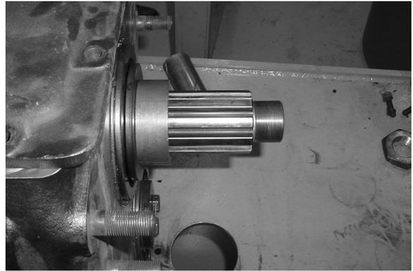
15. Install the rear bearing cover and tighten the capscrews to specifications. Install capscrews in a staggered or opposite sequence.
