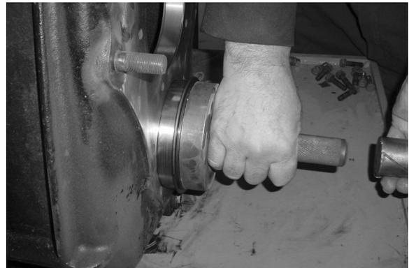
7. Install the rear bearing retainer plate on the rear of the countershaft. Tighten the capscrews to specification and install the lockwire.
