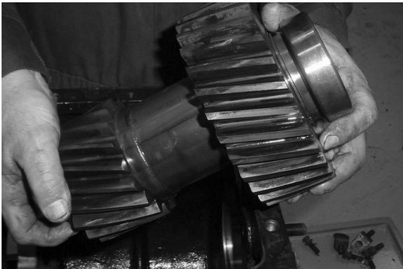
5. Tilt the countershaft and remove through the top of the case.
