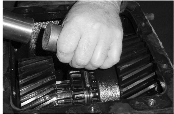
8. Remove the tension spring screw, tension spring, and the tension spring ball from the vertical bore in the right side of the case.
