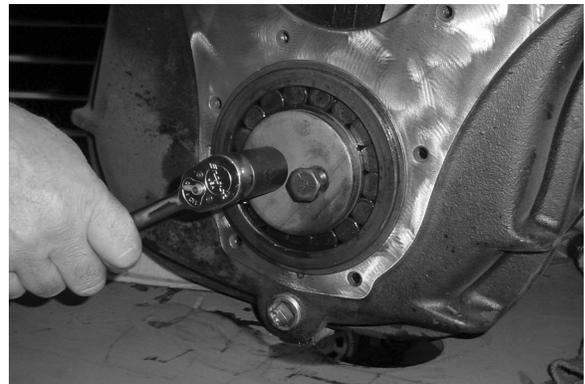
8. Install the front bearing spacer in the front of the countershaft bore.
