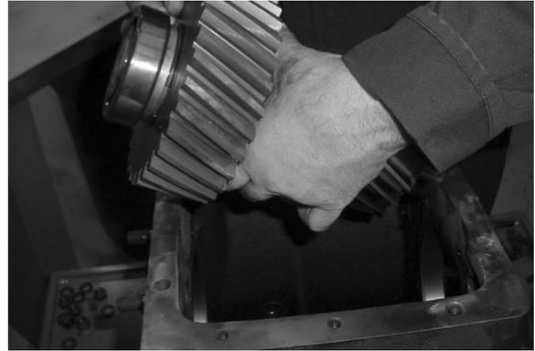
6. Block against the front of the countershaft (not bearing) and install the rear bearing on the shaft. Place into bore.
