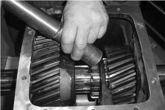
13. Move the mainshaft to the rear, sliding the splined thrust washer forward along the splines of the mainshaft.
