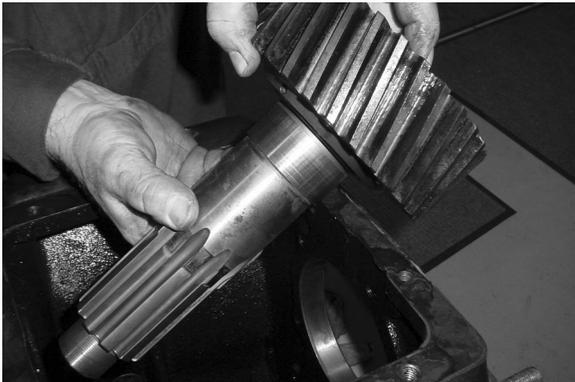
5. Remove the drive gear from inside the case.
