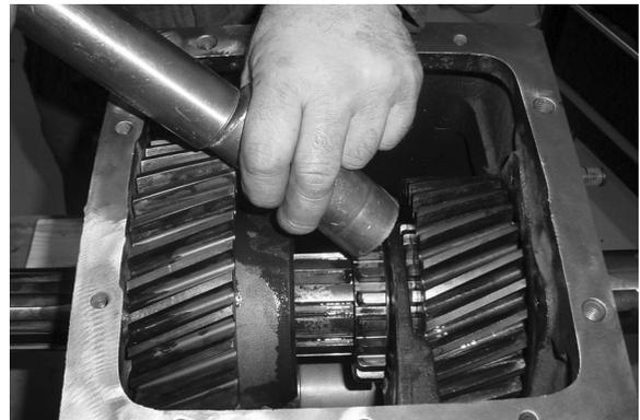
11. Remove the mainshaft key from its keyway between the splines of the shaft.
