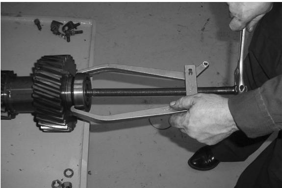
6. Remove the front bearing from the countershaft.
