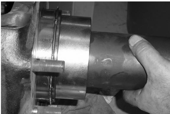
12. Install the mainshaft rear bearing, seating the bearing onto the shaft and into the case bore. When correctly seated the washer between the bearing and gear hub should be tight.
