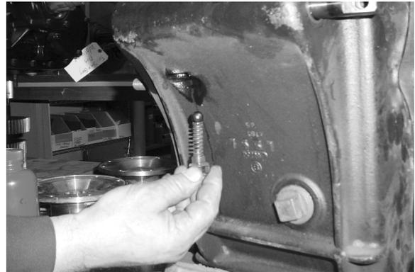
9. Locate the mainshaft washer key which is installed in keyway between the splines of the mainshaft under the sliding clutch gear. Turn the shaft so the key is in the uppermost position.
