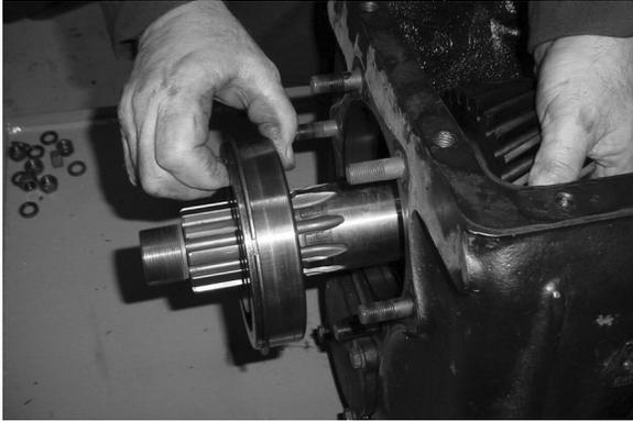
4. Move the drive gear forward to lightly tap the main bearing forward and out of the case bore.
