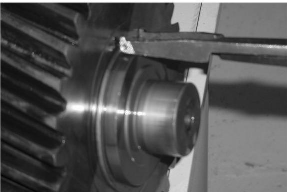
7. Remove the gear retaining snap ring from the front of the countershaft.
