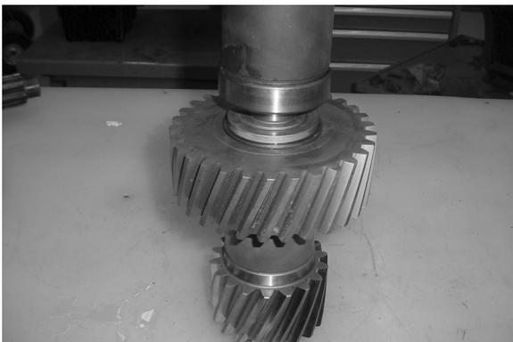
4. Install the front bearing on the countershaft.
