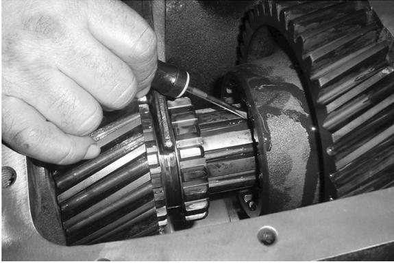
12. Inside the pocket of the low speed gear, turn the splined thrust washer in its groove until the lugs on its inside diameter line up with the grooves in the mainshaft.
