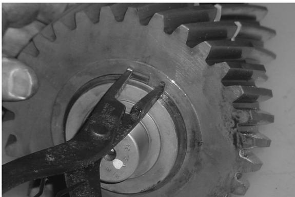
3. Install the snap ring on the front of the countershaft.
