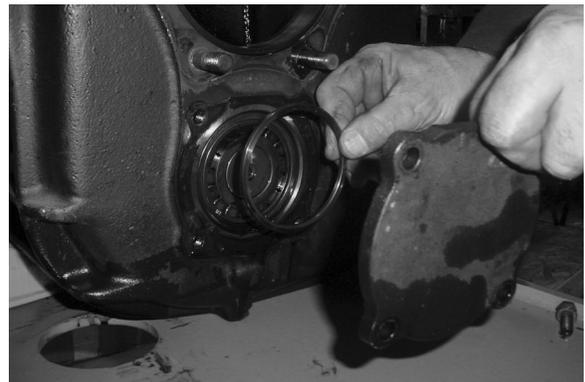
9. Install the countershaft front bearing cover and tighten cap-screws to specifications.
