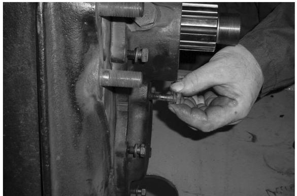
16. If previously removed, install the oil seal in the rear bearing cover. The seal should be flush with the rear face of the cover.
