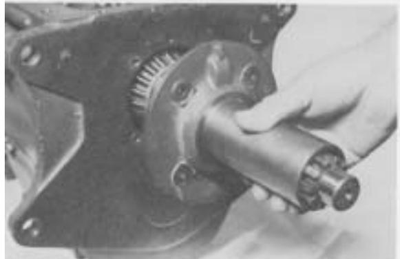
**Figure 159** - Position main drive gear bearing cap on main drive gear. Lube oil groove in cap at the top.
