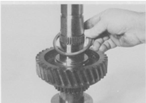
**Figure 35** - Remove 2nd gear split washer retainer ring.
