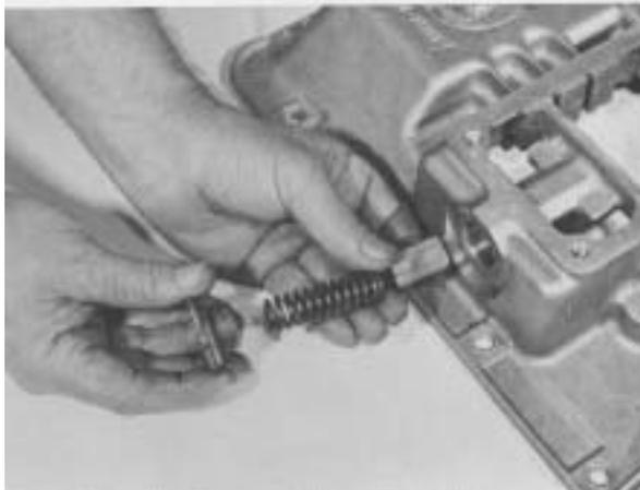
**Figure 118** - Remove reverse latch plunger spring and plunger.
