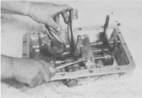
**Figure 82** - Remove front and rear rail support cap-screws.
