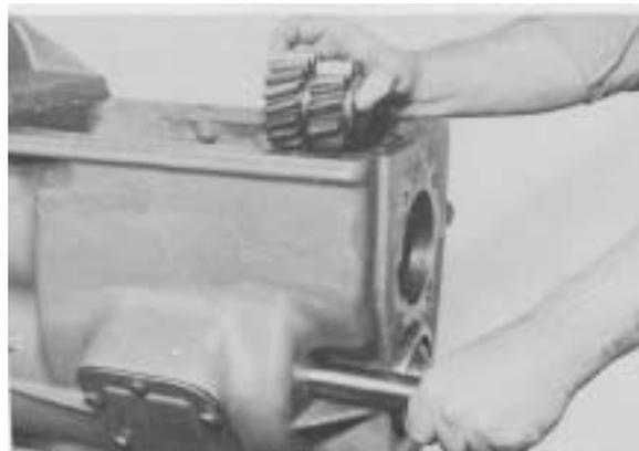
**Figure 13** -Remove reverse idler gear and thrust washers.
