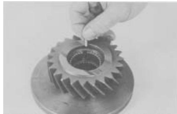
**Figure 69** - Lay up second row of needle rollers.
