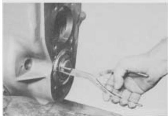
**Figure 14** - Remove countershaft rear bearing retainer ring.
