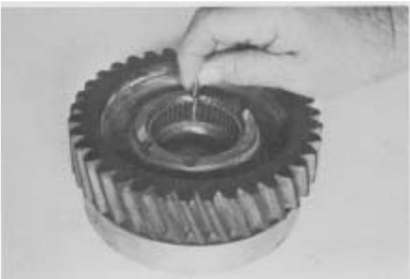
**Figure 48** - Lay up second row of needle rollers.
