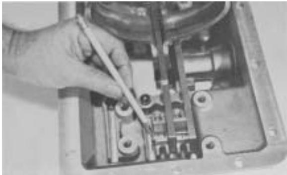
**Figure 128** - Install 2nd interlock tapered pin. Align pin with interlock cross pin hole.
