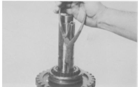
**Figure 32** - Remove 1st & Reverse shift hub sleeve retainner ring.
