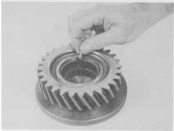
**Figure 40** - Lay up second row of needle rollers.
