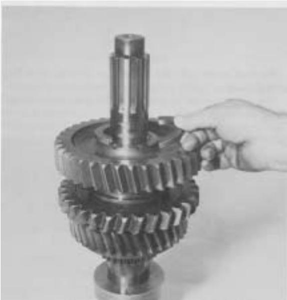
**Figure 30** - Remove 1st gear split washer
