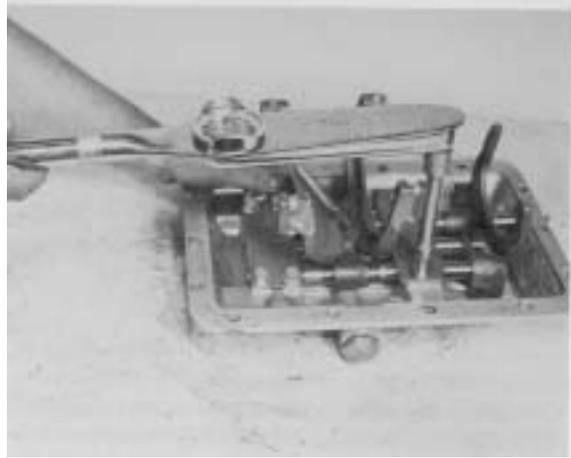
**Figure 102** - Tighten support cap screws 20 - 25 ft.lbs. torque [27,2 - 33,8 N.m].
