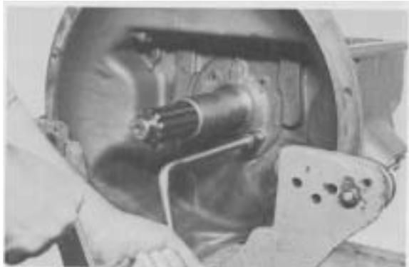
**Figure 6** - Remove main drive gear cap bolts.
