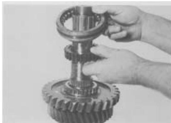
**Figure 33** - Remove shift hub and sleeve.
