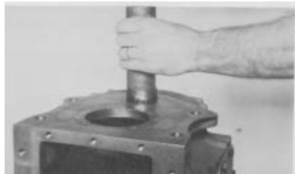
**Figure 81** - If countershaft front bearing is to be replaced, remove clutch housing and drive front bearing from transmission case. Apply a light coat of Loctite 510 on the outer diameter of the new bearing. Install in transmission case as shown with end of bearing .001-.007 below the face of case. Clutch housing is reassembled temporarily on transmission case to facilitate reassembly of transmission, but will be removed again later on to set mainshaft taper bearing end play.
