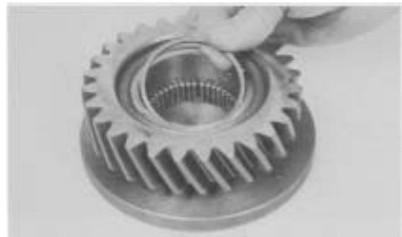
**Figure 39** - Position roller spacer on first row of rollers.
