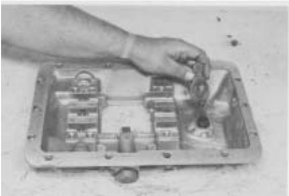
**Figure 89** - Remove 1st & Reverse rocker arm.
