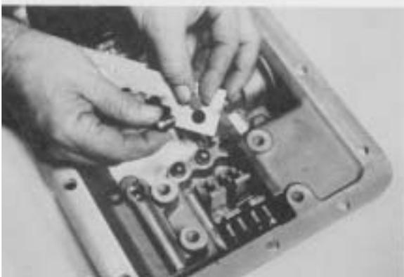
**Figure 112** - Use caution as NOT to lose interlock cross pin, interlock tapered pins or mesh lock poppet balls.
