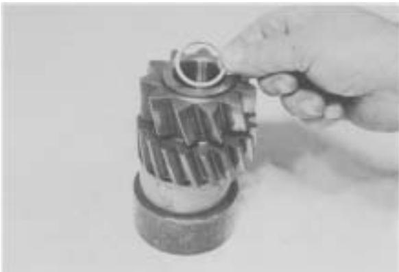
**Figure 146** - Position roller spacer on first row of rollers.
