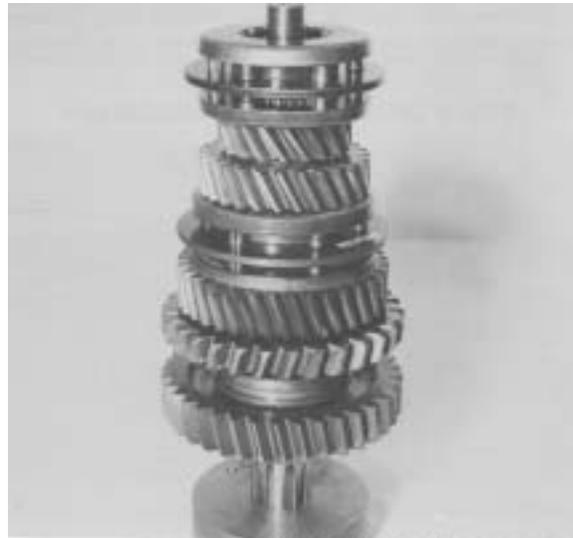
**Figure 75** - Mainshaft assembly complete.
