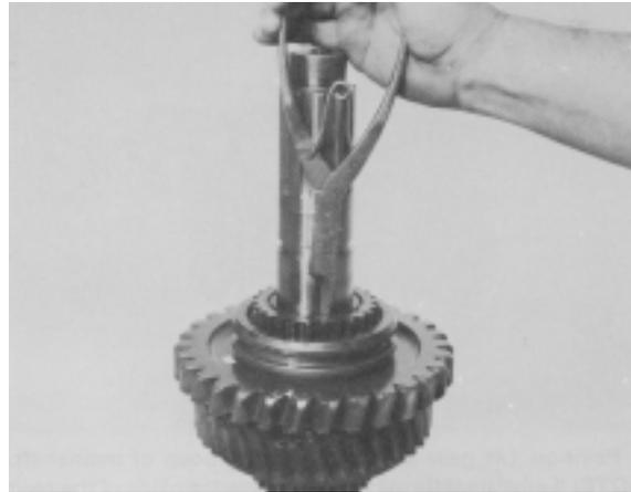
**Figure 61** - Install shift hub sleeve retainer ring.
