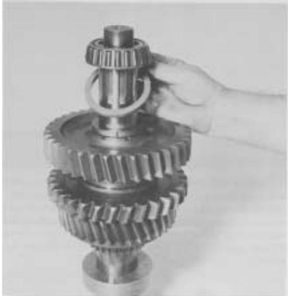
**Figure 29** - Remove rear bearing and split washer retainner ring.
